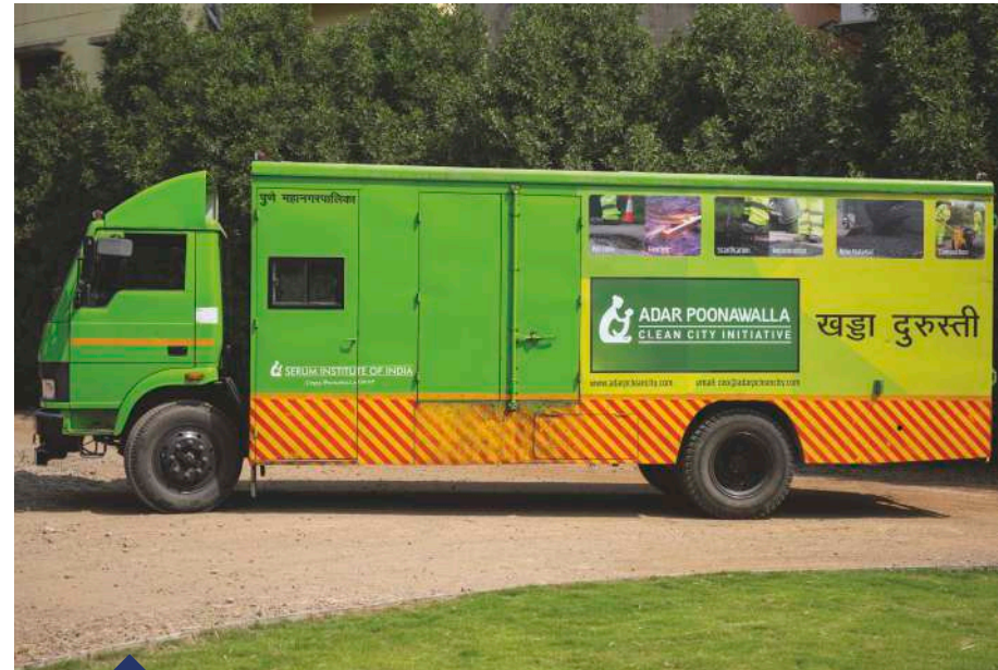
Pothole Repair Machine
